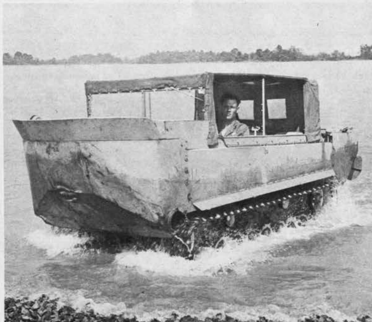
Removable pontoons make the M-29C model look like smaller Dukw. Splash guards protect driver and cargo from water churned by track.
